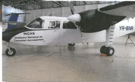
YR - BNR Britten Norman BN-2 Flying lab – Radar & EOS surveillance
